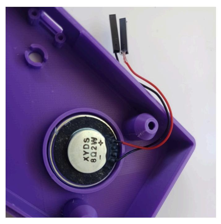
Once the speaker's been prepped, squirt a blob of hot glue into the inner edge of the back case's speaker well and squish the speaker into place - cone side down - on top of it.
