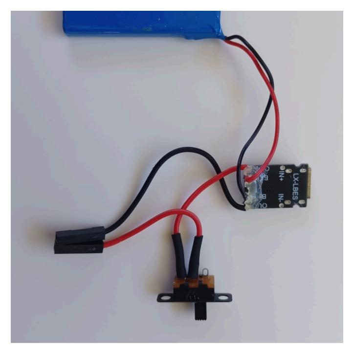
You can now secure the USB-C charger board with two 4mm M2 screws and the LiPo battery with double-sided tape. Drop the slide switch into its cutout near the top-left corner of the back case with the unused tab on the left side.
