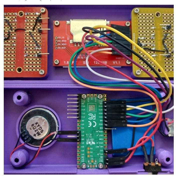
After connecting jumper wires to all the LCD headers, carefully bend the pins over toward the center until they're at a 20-30 degree angle to the board. This will make it easier to close the case later.
