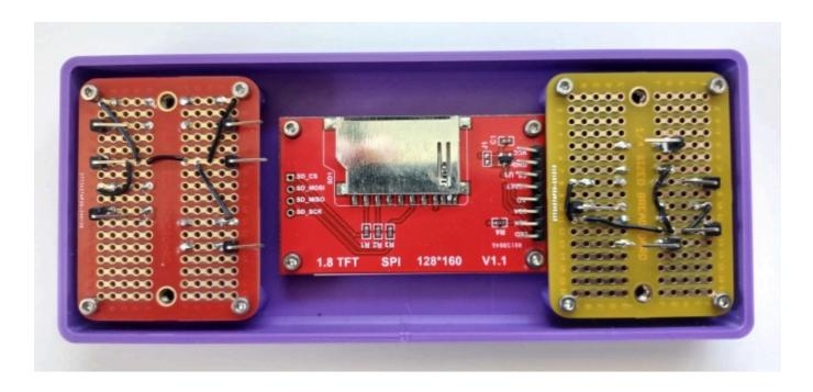
Step 3: Assembling the Back Case
