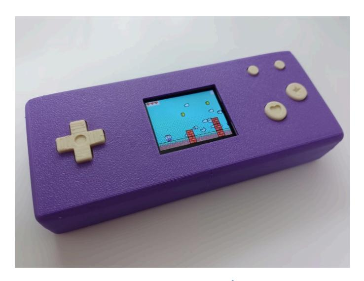
Maketato is a 3D-printed, MakeCode Arcade-compatible handheld that you and your kids can build at home. To keep costs down, it incorporates only cheap, readily-available and reusable parts such as the Raspberry Pi Pico. The enclosure is durable, sized for small hands, and will print quickly and without drama on nearly any 3D printer. Assembly is straightforward enough for a child to perform but not so simplified as to eliminate the possibility of mistakes and the learning that comes from them.
