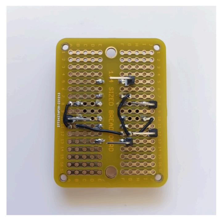
The completed board should like something like the above. If you have a multimeter on hand, it would be good idea to verify that there's continuity between each switch's header pin and the common Ground pin when its button is pressed.
