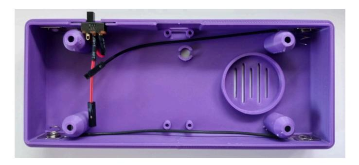
Insert one AA battery into each side of the case, making sure the springs are in contact with the cathodes (or '-' ends) of the batteries.
