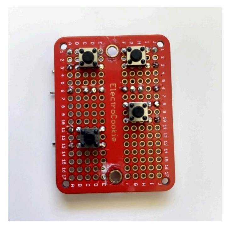
We'll solder an additional header pin in the Ground row on this board, allowing us to daisy chain the Ground from the directional pad PCB and connect all the switches to a single Ground on the Pi. For my build, I soldered a jumper between the left and right sides of row 6 to make an extended Ground row.
