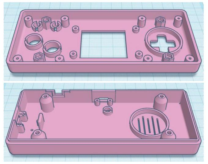
The Maketato's case was designed from the ground up to be durable, easy to print and fit comfortably in small hands. The package I've made available on Cults3D includes STL files for the front and back cases as well as each of the buttons. I've also thrown in an alternative back case design that allows for safer but less convenient AA battery power.
